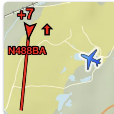
Traffic Warning within 1.3 nm and +/- 1,200' or will be within 25 seconds
